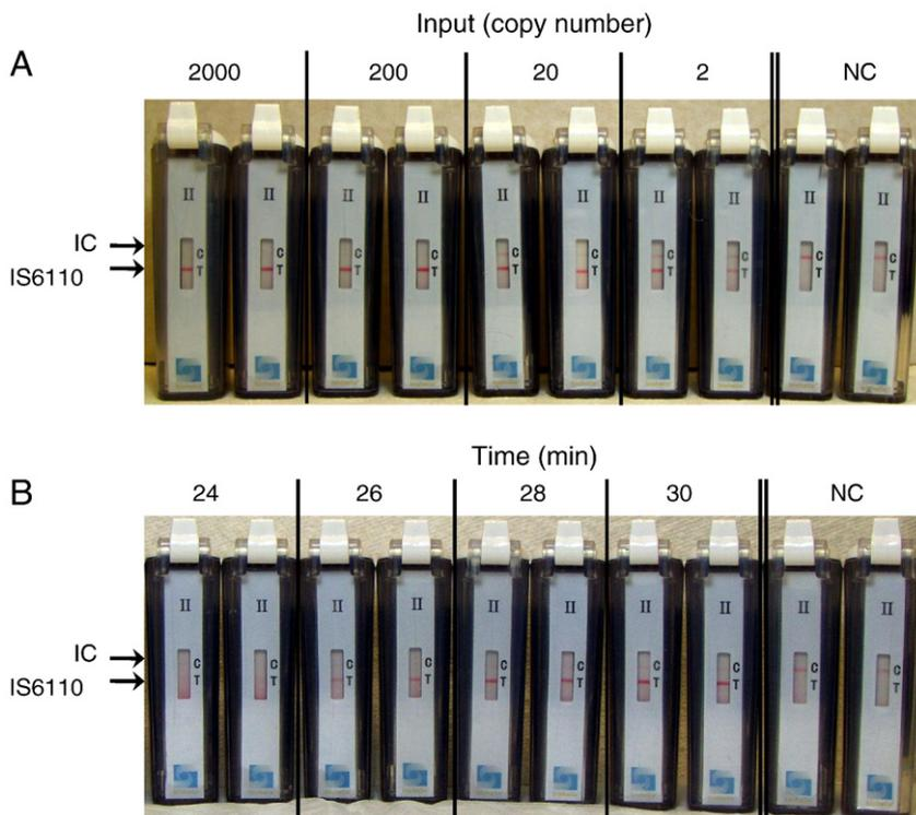
**Fig. 2.** Sensitivity of the HDA-based MTB assay. A. 2000, 200, 20 or 2 copies of gDNA were amplified using the HDA-based MTB assay for 30 min at 65 °C and analyzed by cassette detection. B. 20 copies of gDNA were amplified using the HDA-based MTB assay for 24, 26, 28 or 30 min at 65 °C and analyzed by cassette detection. Each reaction was done in duplicates. Two negative controls (NC) were included in each run and incubated for 30 min at 65 °C.
